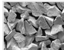
Sintered and Crushed
