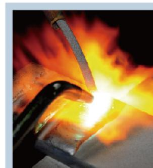
Oxy-Acetylene Flame Welding System
