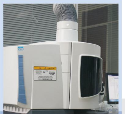
Inductively Coupled Plasma Optical Emission Spectrometer(ICP-OES)
